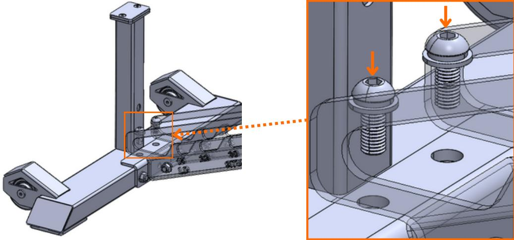
**c. Put on the Small bolt with spring washer and flat washer to the hole on the top of base, Simpy hand tight.**
