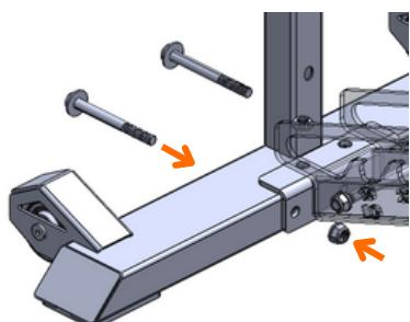
b. Put on the Bolt and washer to the hole and hand tight it with nut. Repeat the process on the other side.
