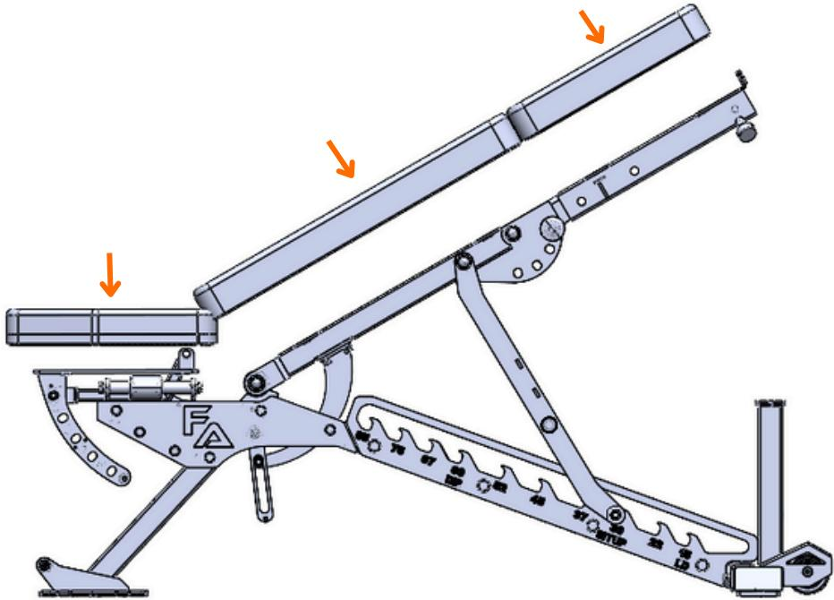
**a. Put on the pads to the Seat, Back and head frame.**
